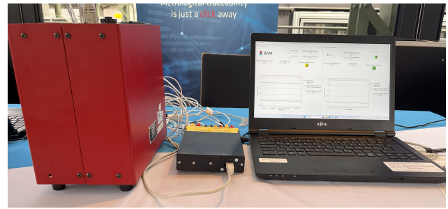
Figure 2. Setup for the demonstrator. The small black box situated centrally within the apparatus contains an Arduino microcontroller. The four temperature sensors are connected to the Arduino. The bigger red box provides a constant temperature of 0 °C for sensors which should measure a stable temperature. The Arduino is connected to the laptop where the demonstrator program is running via USB.
