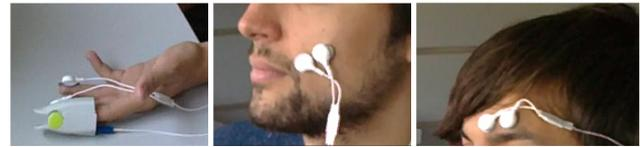
**Figure 4.** Placement of sensors for detecting bio-signals.
