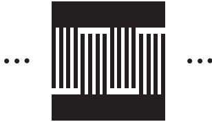
Figure 3. IDT with eight electrodes per period.
