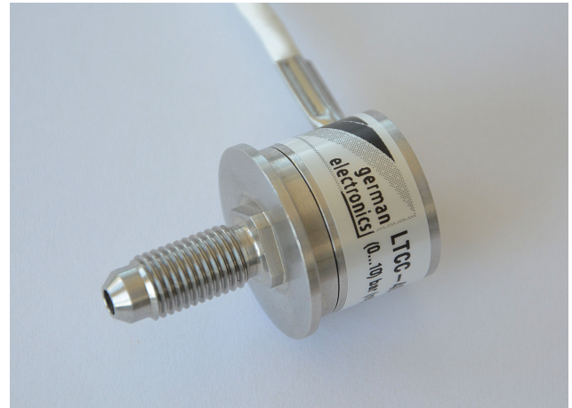
Figure 15. Completely assembled sensor with steel connect screw and welded steel housing with wiring.
